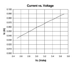
Evaluation Board Data (Vcc=V<sub>BIAS</sub> = 3.0V, I<sub>c</sub> = 56mA) Bias Tee substituted for DC feed inductor (L1)
